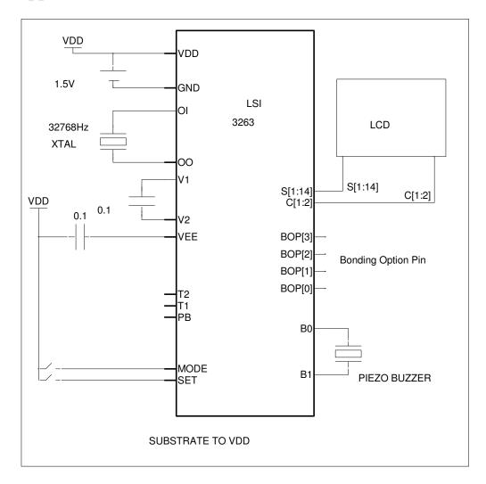
Bonding Option Pin: BOP[0] and BOP[1] to select total numbers of dots:
