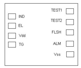
Chip size 1,300 um x 1,050 ms , substrate connected to Vdd
